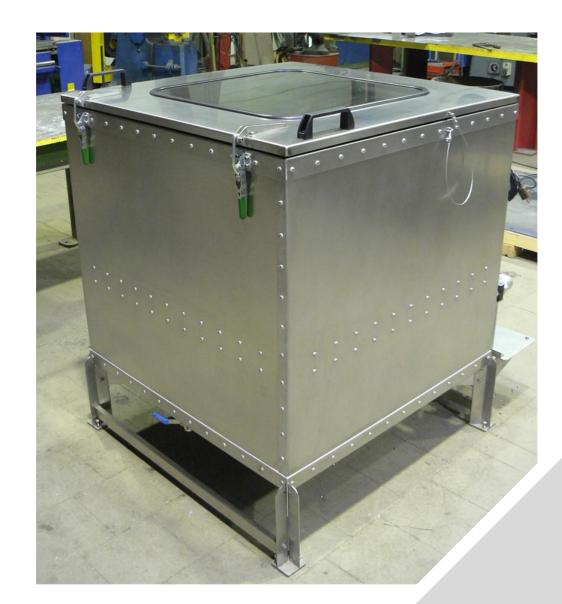
For cleaning medium-sized spray tools, these mobile units are equipped with a swiveling hood featuring integrated all-around viewing windows.
