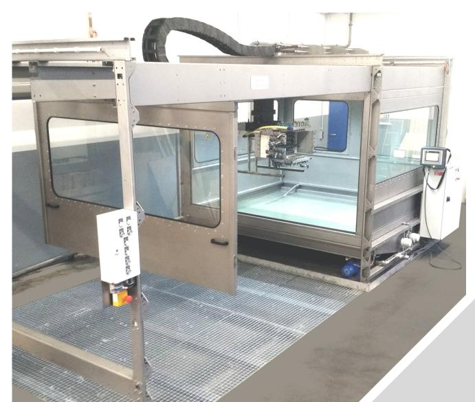
This cleaning system is designed for very large and heavy spraying equipment. Thanks to the drivability of the station, the spraying equipment can be positioned safely and easily.
